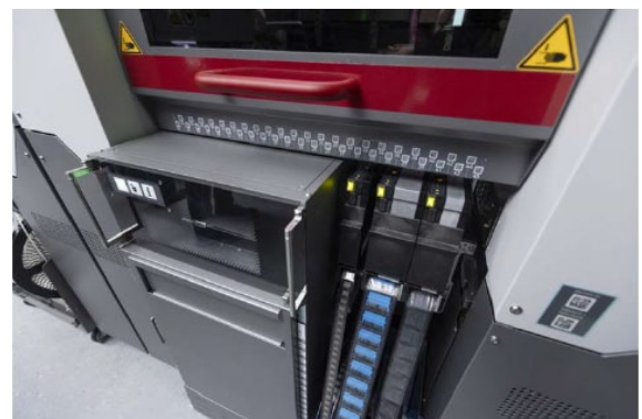
Combination of tray unit and odd-shaped component feeder: The SIPLACE V platform offers maximum flexibility for demanding high-mix production requirements. (Image credit: ASMPT)
