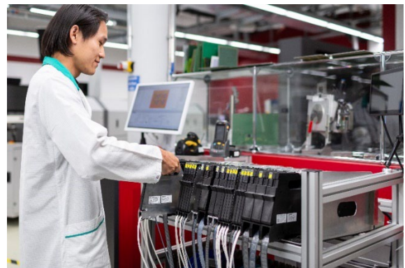
WORKS Logistics organizes and optimizes the intermediate storage of material in an Active Feeder Rack in the setup preparation area. (Image credit: ASMPT)
