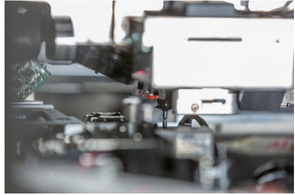
Flip chip unit: Four flip nozzles detach the dies from the wafer's carrier foil and transfer them to a buffer system. This process, which runs parallel to the placement process, increases the processing speed significantly. (Image credit: ASMPT)
