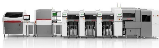
A continuous high-speed SiP production line: A DEK Galaxy solder paste printer followed by the Process Lens SPI system, fast SIPLACE TX micron placement machines and the hybrid SIPLACE CA2 at the end of the line, which also places dies directly from the wafer. (Image credit: ASMPT)
