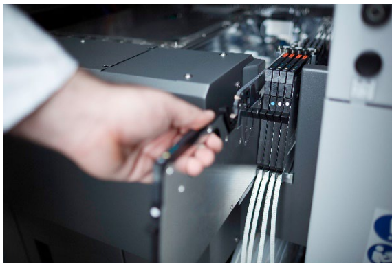
Supplied via a feeder, the SIPLACE CA2 also processes classic SMT components such as resistors, capacitors, transistors and diodes at speeds of up to 76,000 cph. (Image credit: ASMPT)
