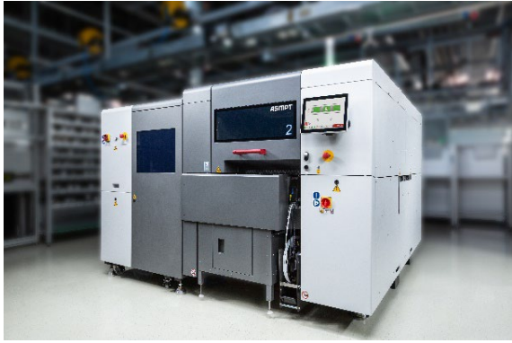
The hybrid SIPLACE CA2 brings two worlds together in one machine: conventional SMT assembly and pioneering advanced packaging in a footprint of just 2.56 by 2.50 meters (L x W). (Image credit: ASMPT)
